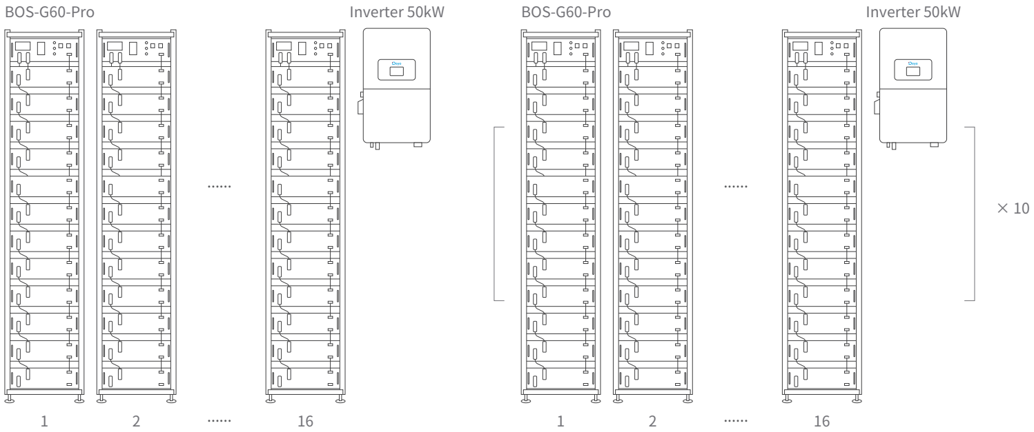
Maximum support for 16 racks of batteries in parallel
