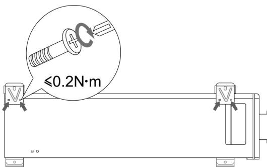
3) Stack the battery one by one and then secure them with 4 bolts (M4\*12). The number of stacked batteries can not exceed 6.
