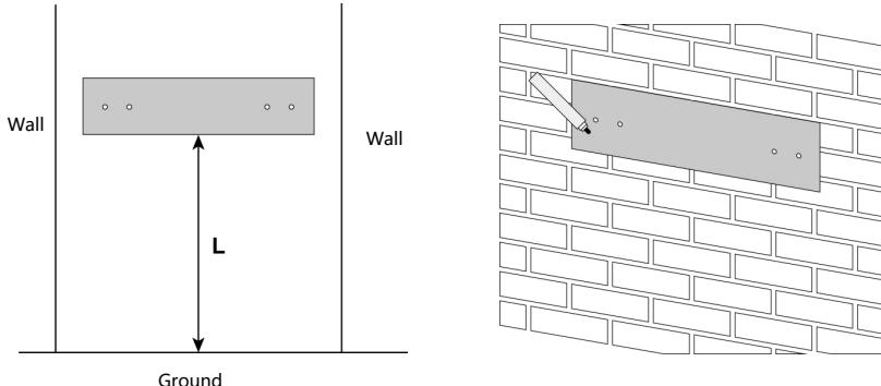
How to differ the floor-mounted installation from the wall-mounted installation depends on the **clearance L** between the ground and the positioning cardboard.
