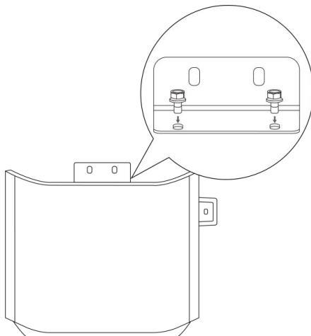
4. Secure batteries to the wall using 2 expansion bolts (M6).
