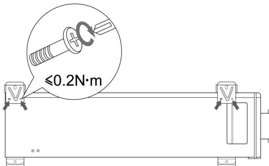
3) Stack the battery one by one and then secure them with 4 bolts (M4\*12). The number of stacked batteries can not exceed 6.
