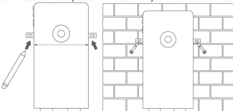
3) Adjust the left and right screws to the appropriate position to ensure that the battery is perpendicular to the ground.
