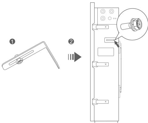
2) Make the back side of the battery close to the wall, and then mark locations of two assembly holes. Drill two holes and secure the battery to the wall in the same way as mentioned above in 4.3.1.
